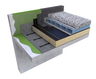
It is recommended for use as part of a warm roof system as this will ensure the designed thermal performance of the flat roof is maintained.
