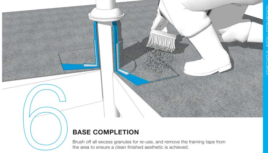
Broadcast, by hand, coloured mineral granules to suit the existing or new roof finish. STARCOAT® R is UV stable so can be left exposed without a granular finish if required.
