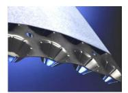
High compressive strength, rigid HDPE board acting as both drainage and water retention layer, with a geotextile filter layer bonded to one side. The board is dimpled and contains high capacity dimples (height approx. 20mm) for water retention and perforations to drain surplus water. It is resistant to root penetration and to chemicals.
