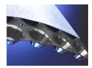
High compressive strength, rigid HDPE board acting as both drainage and water retention layer, with a geotextile filter layer bonded to one side. The board is dimpled and contains high capacity dimples (height approx. 20mm) for water retention and perforations to drain surplus water. It is resistant to root penetration and to chemicals.
