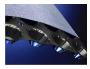
High compressive strength, rigid HDPE board acting as both drainage and water retention layer, with a geotextile filter layer bonded to one side. The board is dimpled and contains high capacity dimples (height approx. 20mm) for water retention and perforations to drain surplus water. It is resistant to root penetration and to chemicals.
