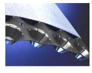
High compressive strength, rigid HDPE board acting as both drainage and water retention layer, with a geotextile filter layer bonded to one side. The board contains high capacity dimples (height approx. 20mm) for water retention and perforations to drain surplus water. It is resistant to root penetration and to chemicals.
