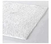
Expected durable service life of the material is up to 50 years in soils with  $4 \le pH \le$  9 and soil temperatures  $\le 25^{\circ}$ C, based on a durability assessment.
