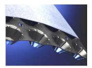
High compressive strength, rigid HDPE board acting as both drainage and water retention layer, with a geotextile filter layer bonded to one side. The board contains high capacity dimples (height approx. 20mm) for water retention and perforations to drain surplus water. It is resistant to root penetration and to chemicals.
