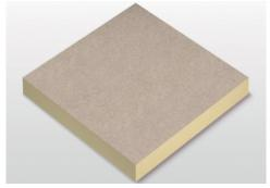
Hytherm LQ comprises a high performance rigid thermoset PIR fibre free insulation core. The board is manufactured with a coated glass tissue-based facing bonded to the insulation core during manufacture. Its thermal conductivity is as low as 0.028 W/m·K and compressive strength is high, typically exceeding 400 kPa at 10% compression.
