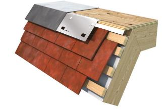
For membrane and liquid applied roof coverings, a suitable metal flashing material should be used to cover the ventilator welting around the lower edge and extending onto the roof to facilitate a lap joint in accordance with the manufacturer's instructions. These flashings should not be installed in lengths exceeding 1m and have a minimum lap of 150mm at the joints.
