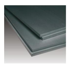
The insulation boards are grey with a smooth skin on both surfaces. Infra-red particles are finely dispersed and incorporated into the extruded cell walls. These lead to reduced heat transfer to keep a building warm in winter and cool in summer.
