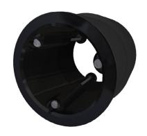
Select the correct seal size prior to installation by measuring the internal diameter of existing pipework. The seal should be inserted into the outlet stem and the stainless steel screws tightened using the Mechanical Seal installation tool, also available from Axter Ltd, until the top half of the seal has expanded. The whole component is then placed into the new or existing roof drainpipe.
