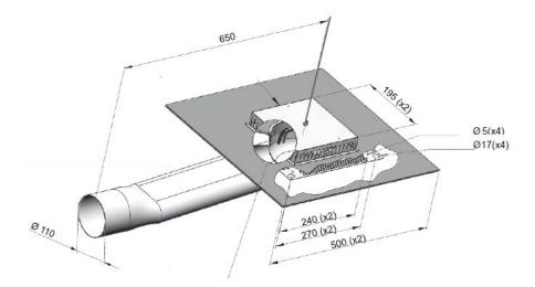
A minimum of 2 outlets is required (regardless of the roof size) with water depth of 35mm.
