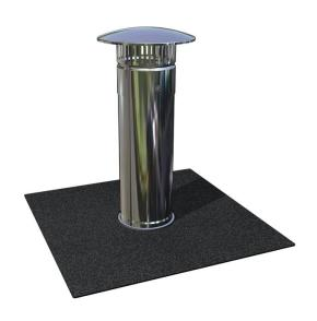
Used on flat roofs with either bitumen or single-ply systems, the Stainless Steel SVP Cover is supplied with a square factory-fitted flange to match the specific membrane being used, thereby providing an excellent bond.
