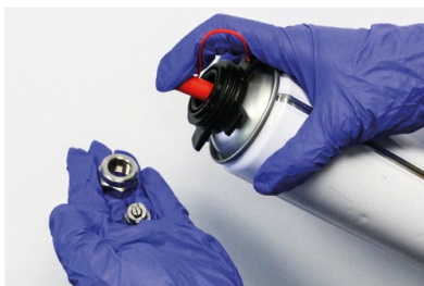
Image 8 Clean with Cleaning Aerosol.
