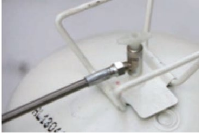
Image 1: Canister with the braided-hose attached properly.
