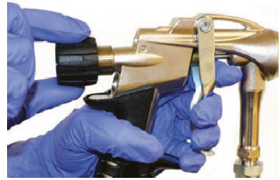
Image 4: Black valve to adjust spray pattern.
