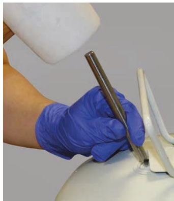
Image 17: Pierce disk at perimeter
