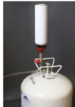
Image 10: Screw Cleaning Aerosol into the adaptor
