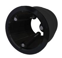
Select the correct seal size prior to installation by measuring the internal diameter of existing pipework. The seal should be inserted into the outlet stem and the stainless steel screws tightened using the Mechanical Seal installation tool, also available from Axter, until the top half of the seal has expanded. The whole component is then placed into the new or existing roof drainpipe.
